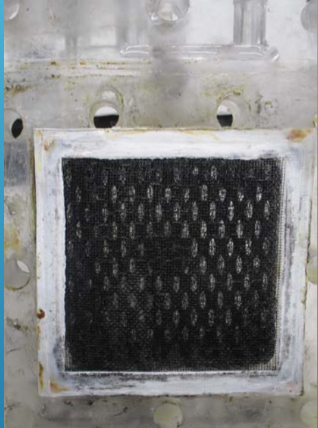
↑ Showing COS deposited on ALL cathode surfaces.
