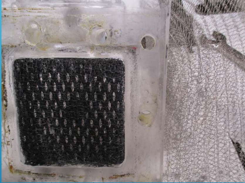
↑ Bare nickel cushion layer ↑ Showing COS deposited on cushion layer and current collector.
